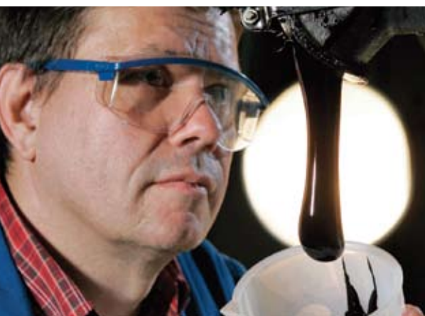
At Imperial Oil's research center in Calgary, technologist Karl Pustanyk demonstrates how thick Alberta's heavy oil is. "Now you see why we have to use steam," he says.
